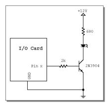
Figure 1: Basic transistor switch
