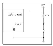
Figure 3: Reading a switch
