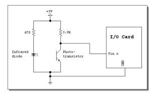
Figure 4: Open-collector circuit
