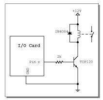
Figure 2: Driving a relay
