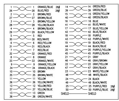
30AWG except two 28AWG pairs where noted as 28# above
